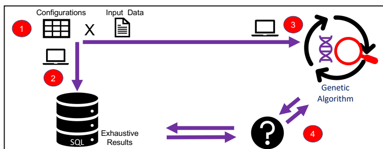
Fig. 1. Overview of the FRDDE framework. It starts with a set of configurations and input data (#1) and populates the database (#2). A genetic algorithm can then be run #3 and the database can be used to answer questions #4.
