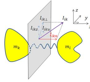
Fig. 3: Impulse decomposition along normal and tangential directions.
