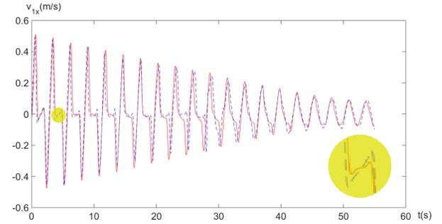
Fig. 5: Time trajectories of the horizontal velocity of Newton's cradle: experiment (red line) vs. simulation (blue dashed line).
