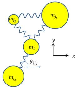
Fig. 1: Contact modeling with virtual springs.
